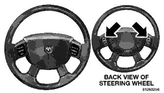
The right hand control is a rocker type switch with a button in the center. Pressing the top of the switch will increase the volume and pressing the bottom of the switch will decrease the volume. The center button of the right hand control will allow you to change the mode.
